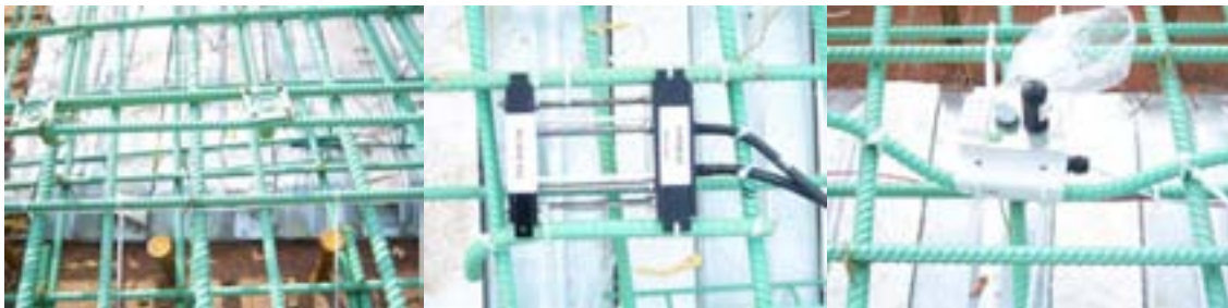
Three Types of Sensors Installed During Phase I: Vetek, CPMP, and EC11 (Embedded Corrosion Instrument).
