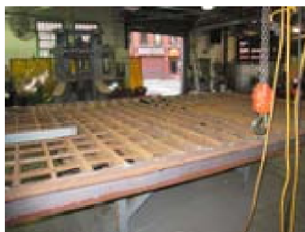
New Grizzly Under Fabrication for the Agency Hamilton Asphalt Plant. (Credit: Russell Holcomb)
