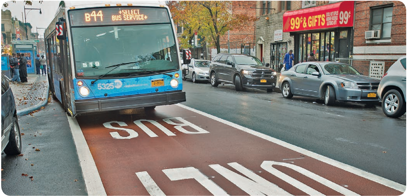
B44 SBS in offset bus lane leaving bus bulb station
