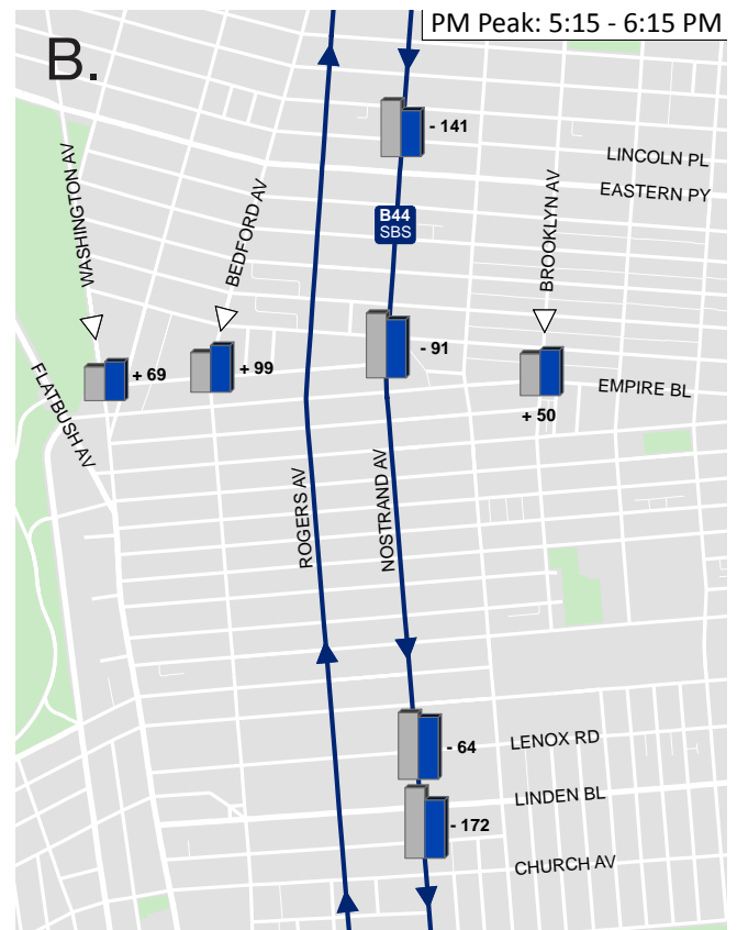
Southbound volume change on Nostrand and parallel streets at Empire Boulevard in the (a) AM Peak and (b) PM Peak
