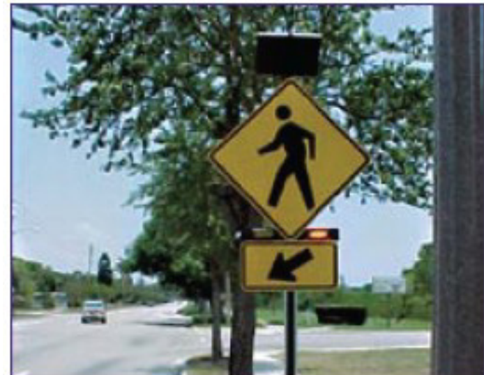
A Rapid Response Flashing Beacon (Image source: Federal Highway Administration)
