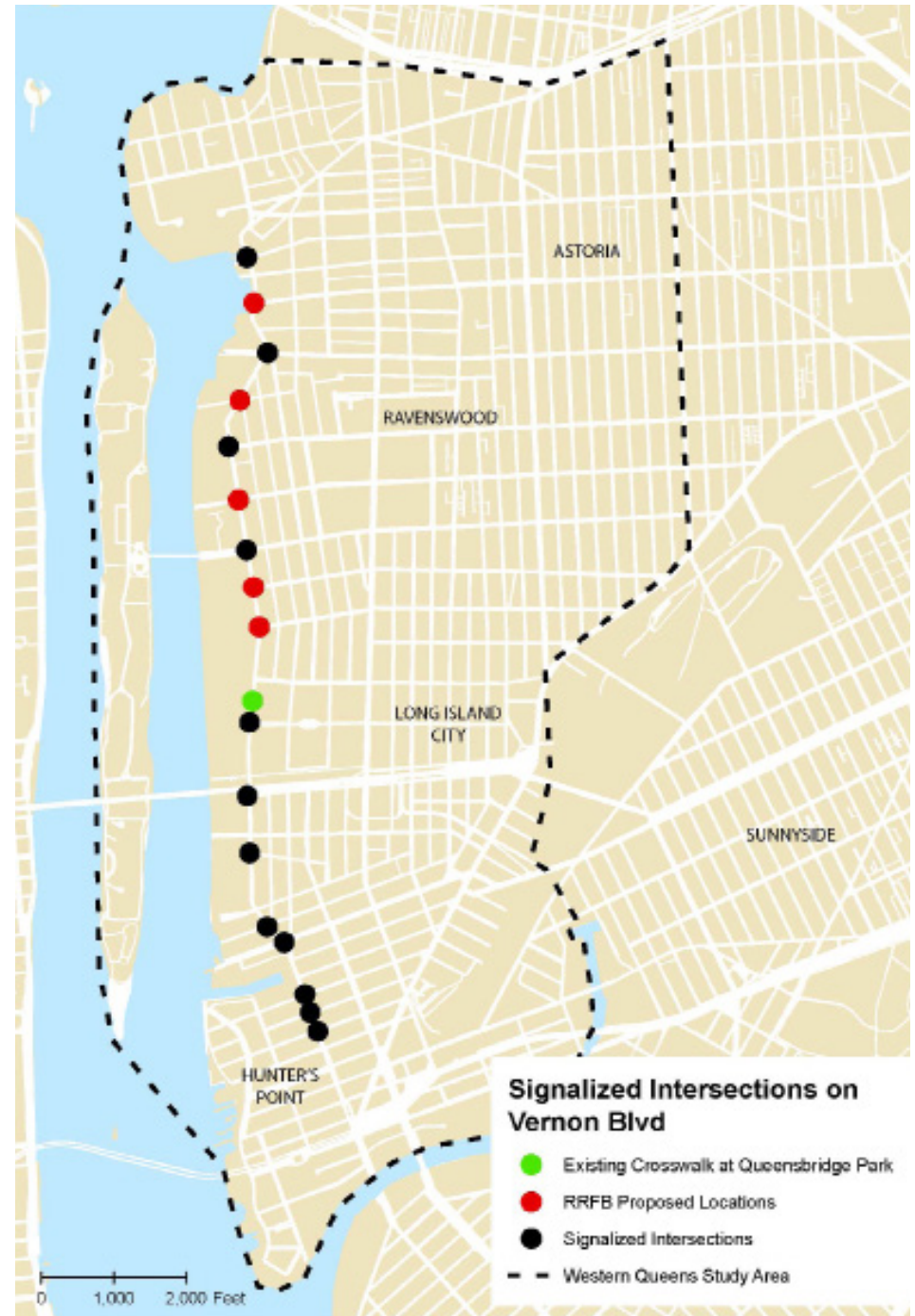
Recommended Rapid Response Flashing Beacon Locations
