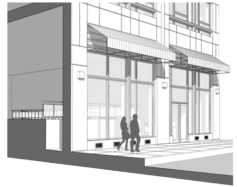
Hybrid floodproofing strategy with commercial display space closer to the pedestrian level
