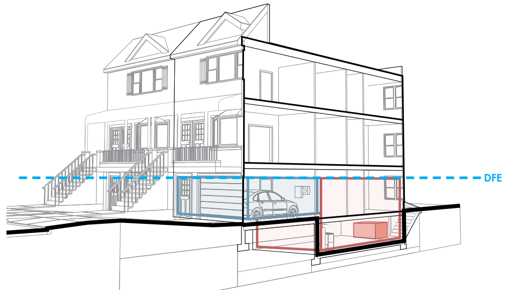
Floodproofed mechanical systems (shown in red) in place, floodproofed garage (shown in blue)
