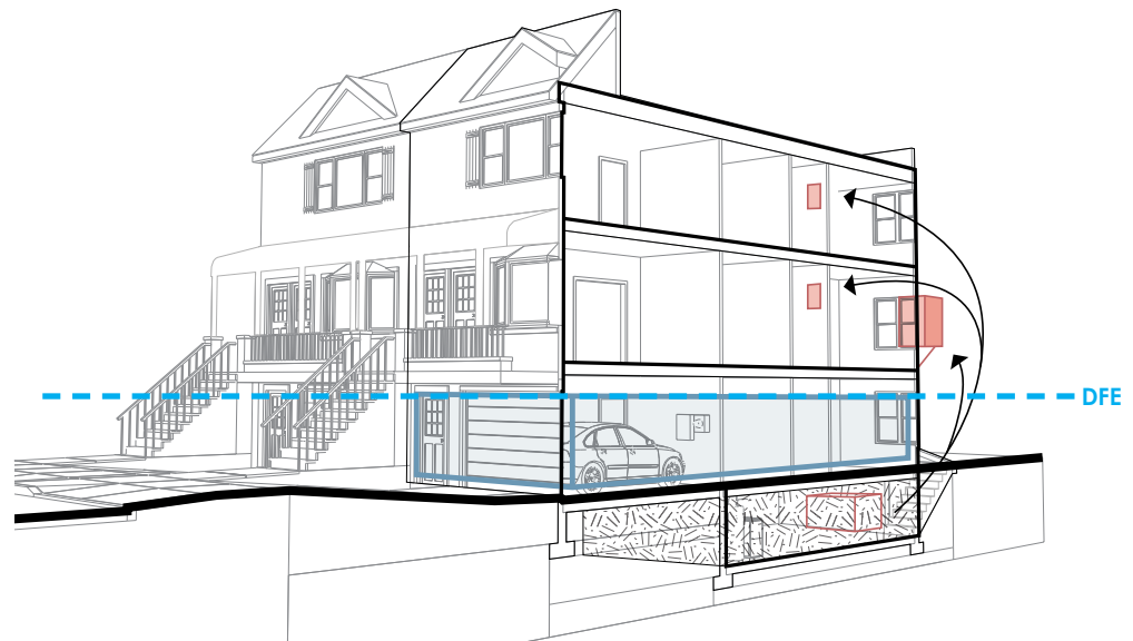
Floodproofed ground floor (shown in blue) in place, Filled in basement and elevated mechanical systems (shown in red) above the DFE
