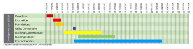
Figure 20-2 Jamaica Prototypes Sample Construction Schedule – 25,000-75,000 sf Development
