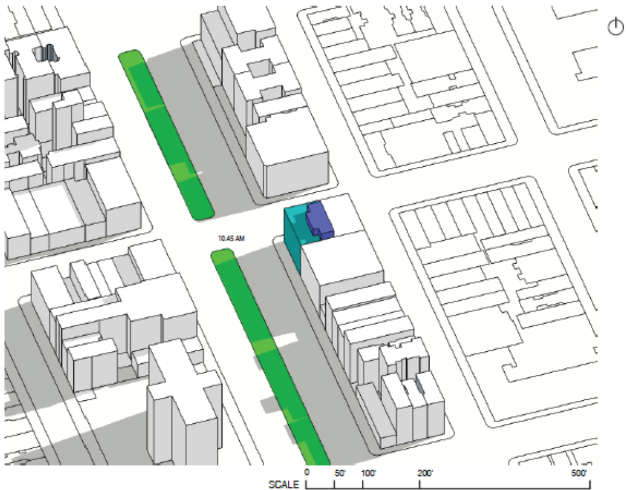
Figure 2.2-9: Tier 3 Screening Assessment Incremental Project-Generated Shadows with Shadows from Intervening Buildings on the May 6 th /August 6 th Analysis Day
