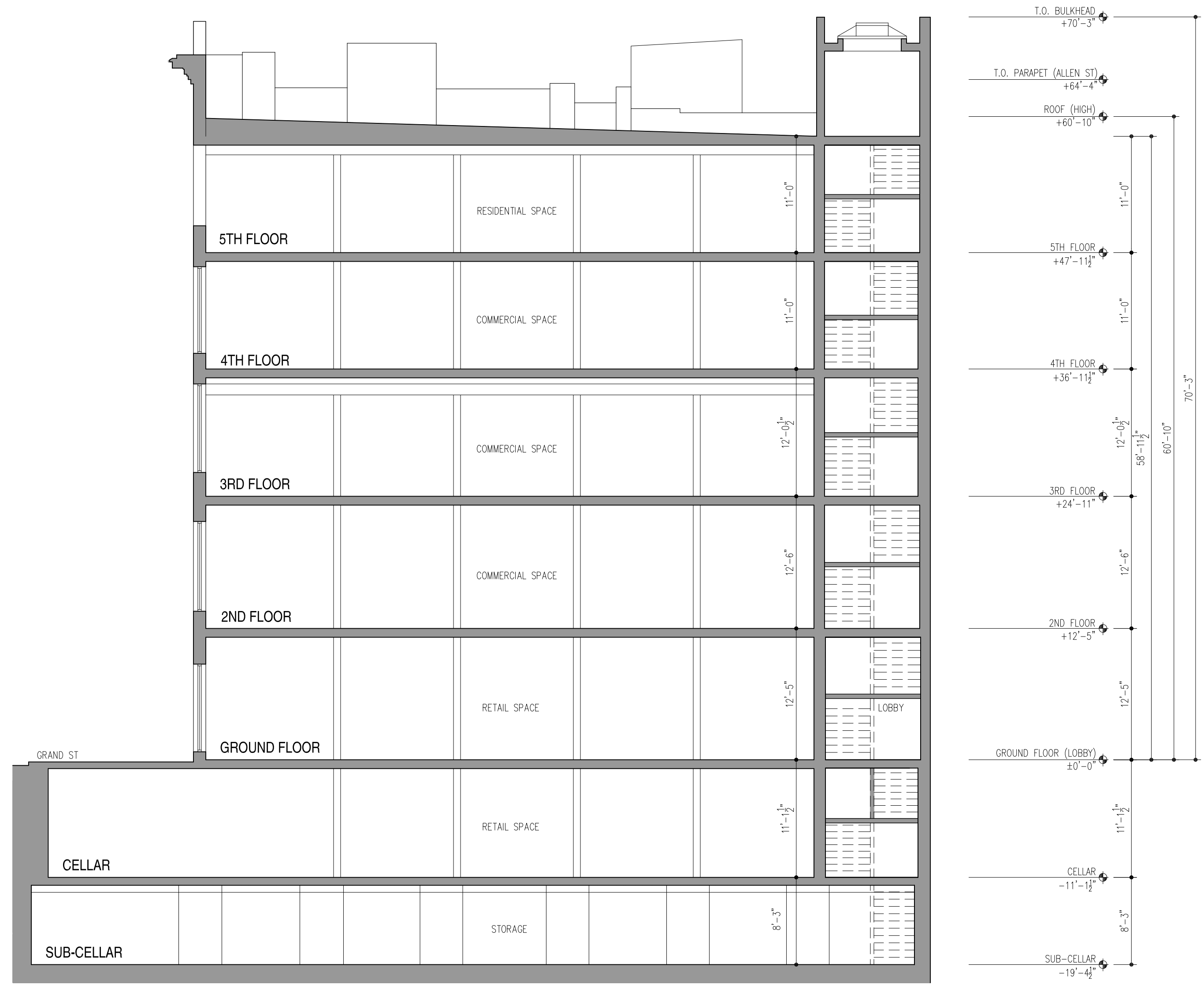
1 EXISTING LONGITUDINAL SECTION A301 1/4"=1'-0"
