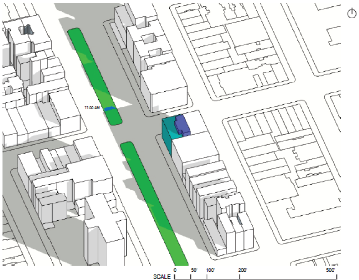
Figure 2.2-5: Tier 3 Screening Assessment Incremental Project-Generated Shadows with Shadows from Intervening Buildings on the December 21 st Analysis Day
