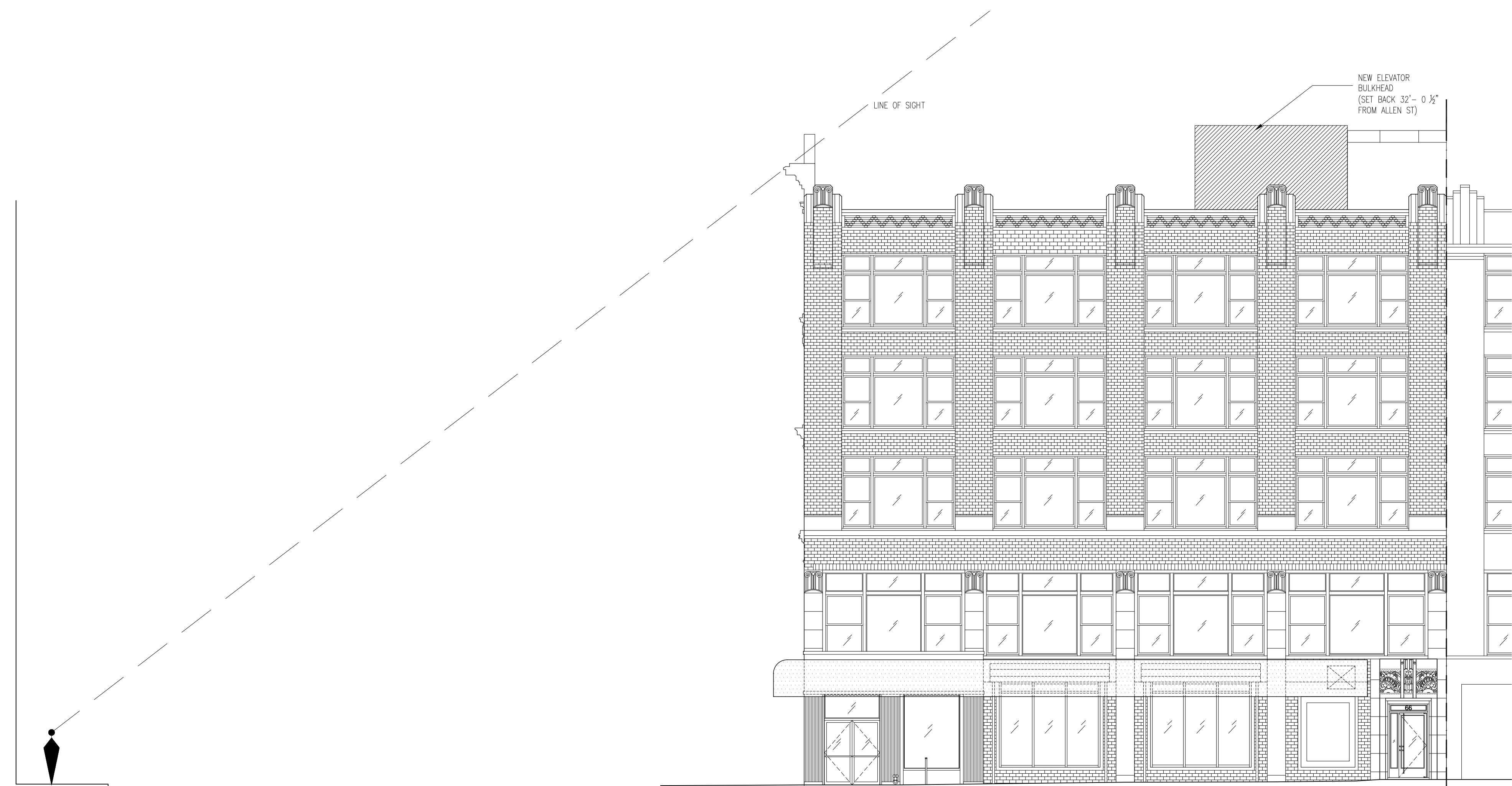
1 GRAND ST: SIGHT LINE DIAGRAM A202 1/8"=1'-0" PROPOSED ELEVATOR BULKHEAD NOT VISIBLE ACROSS GRAND STREET
