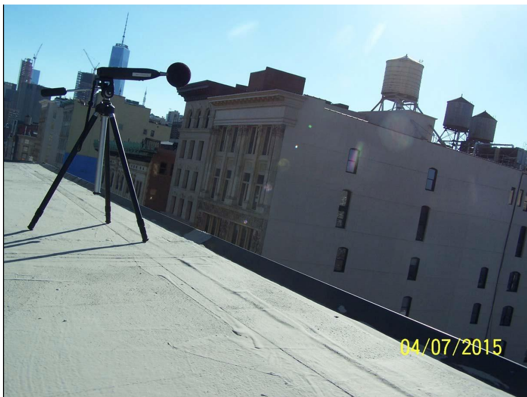
Photo 2: Placement of meter at edge of roof at Broadway frontage; direction looking: Southwest
