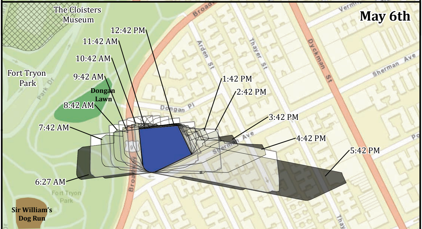
FIGURE 15: TIER 3 SHADOW SCREENING ASSESSMENT FOR MARCH 21st AND MAY 6th (14-story No-Action)
