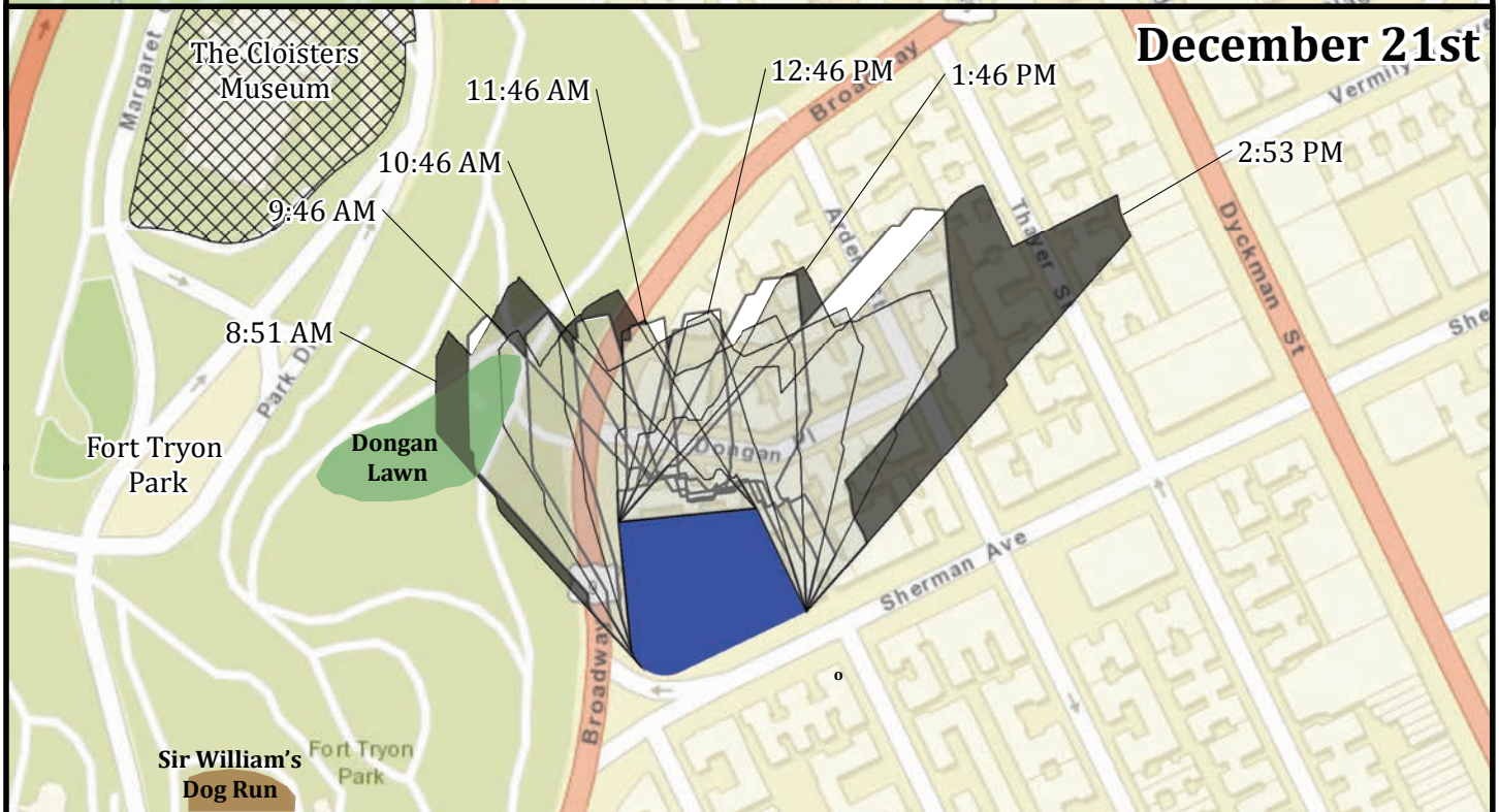
FIGURE 17: TIER 3 SHADOW SCREENING ASSESSMENT FOR JUNE 21st AND DECEMBER 21st (14-story No-Action)
