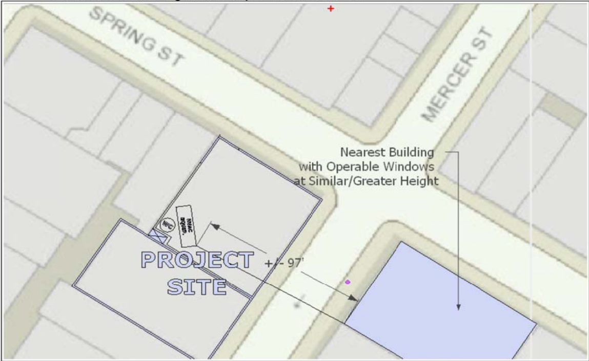
Exhibit 5: Nearest Building with Operable Windows of Similar/Greater Height
