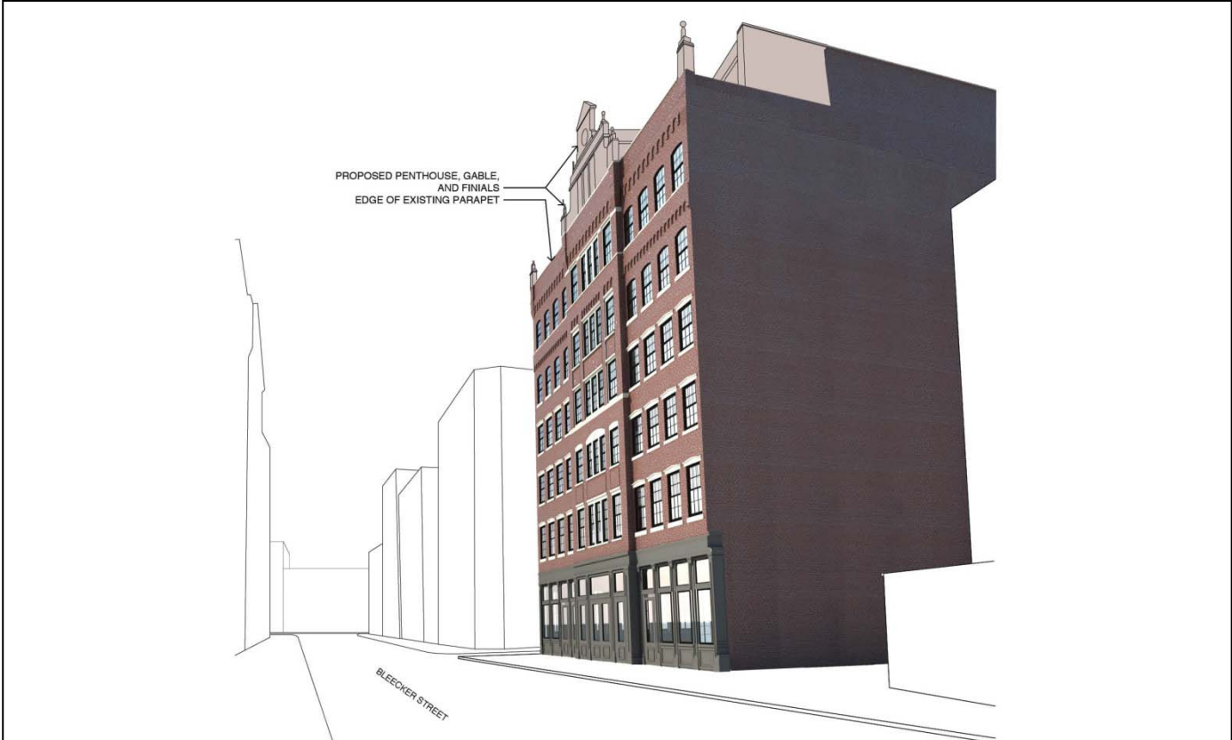
2 Rendering of the Proposed Conversion and Rooftop Additions (new structures shown in gray)
