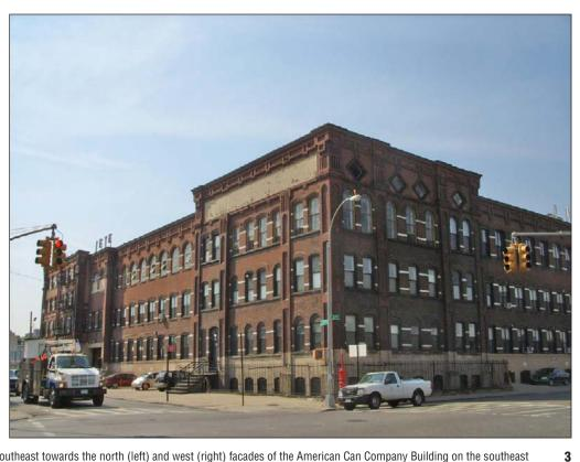
Looking southeast towards the north (left) and west (right) facades of the American Can Company Building on the southeast corner of 3rd Street and 3rd Avenue. Note the segmental-arched windows, corbelled brick cornice, and multi-light diamond-shaped windows on the upper story of the west façade
