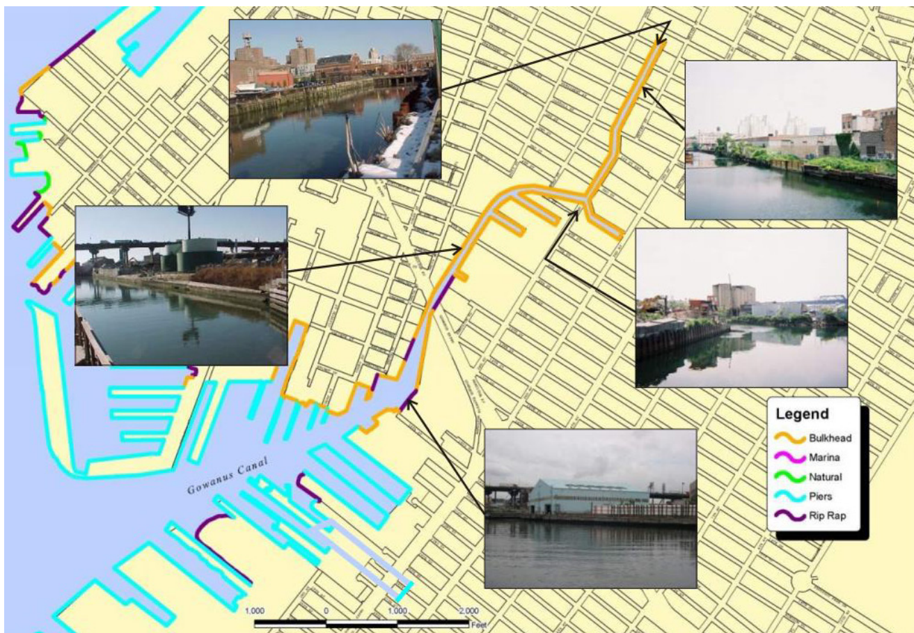
FIGURE 2-4 Existing Physical Characteristics of Gowanus Canal Shorelines (Source: NYCDEP, Gowanus Canal Waterbody/Watershed Facility Plan, 2008)
