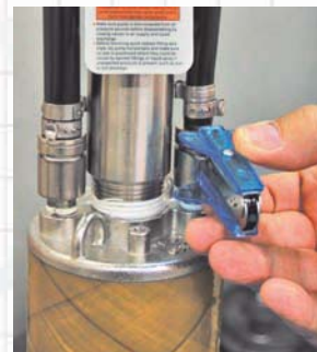
Pull out the release clips.
