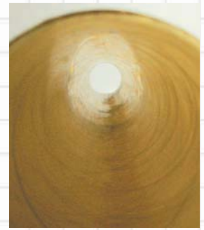
Smooth ID helps reduce the rate of solid buildup inside the casing.
