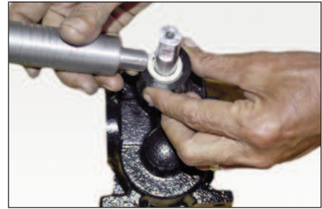
Fig.11. Installing gasket using pipe assembly
