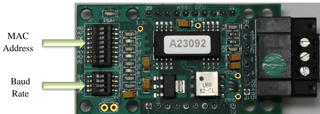
Figure 17. BACnet MS/TP Switches
