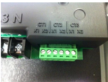
CT Terminal Block in Place
