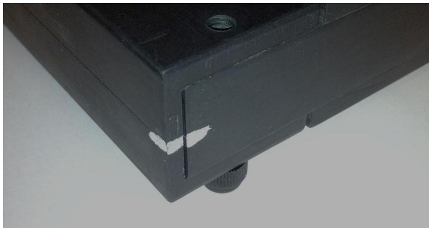
Figure 7: Hash Marks on Split Core CT
