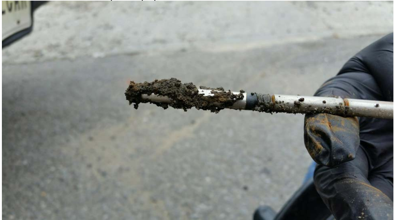
Photo 1: water level meter probe tip upon retrieval from MW-05.
