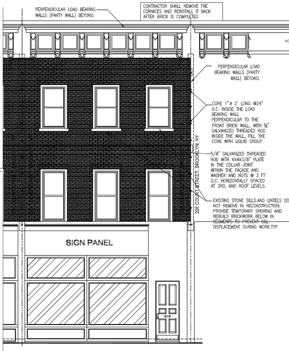
1 S-101 TYING THE WALL TO THE FLOOR DIAPHRAGM SCALE: 1/2"=1'-0"
