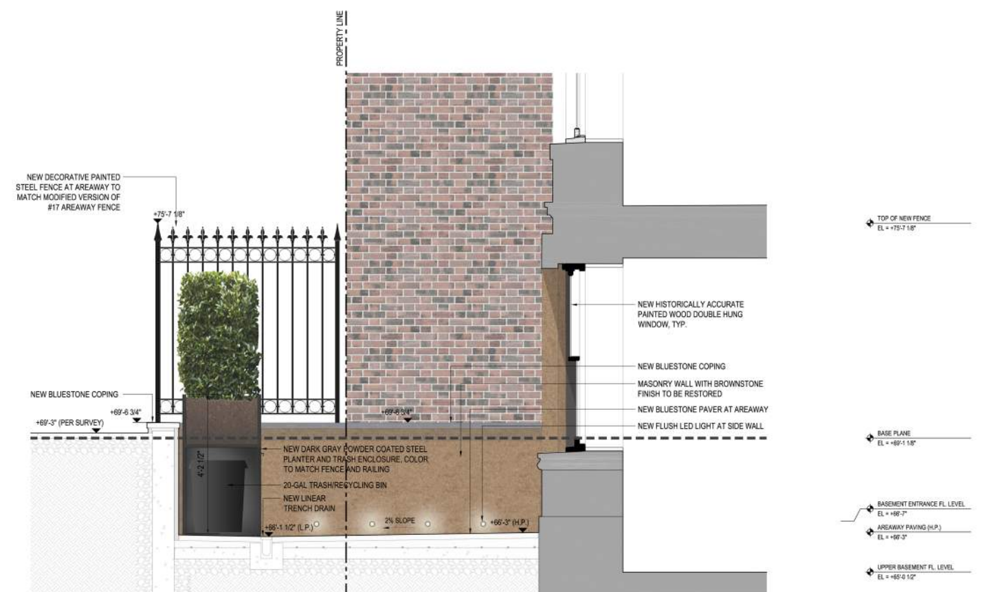
Areaway: Proposed Section at 15 E77th Street
