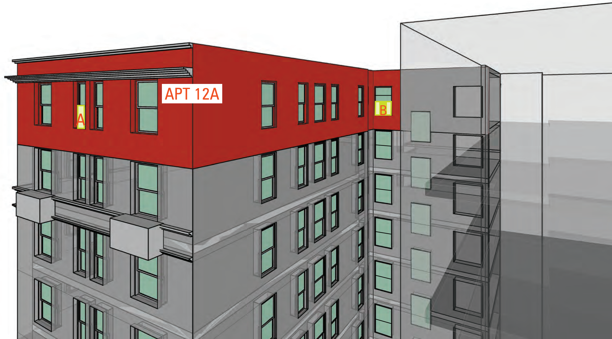
A - CONDENSING UNIT AT LOWER HALF OF WINDOW WITH AWNING UNIT ABOVE B - CONDENSING UNIT AT LOWER HALF OF WINDOW WITH DOUBLE HUNG ABOVE TO MATCH 4TH FLR INSTALLATION
