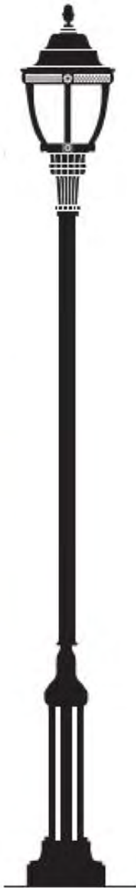
NYC DOT STANDARD TYPE "B" LAMP NEW LIGHTING TO MATCH EXISTING
