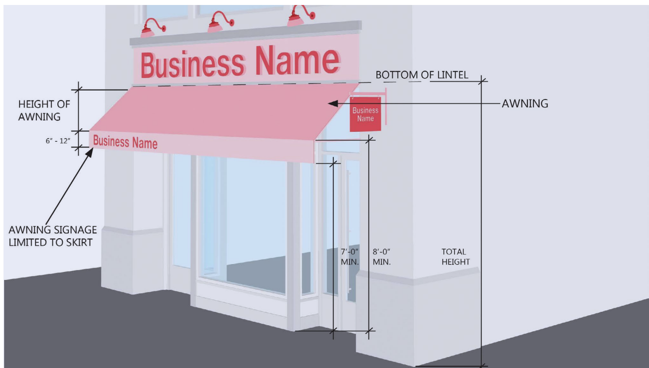
Typical storefront awning location and dimensions.
