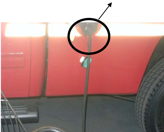
Defueler hose in diesel gas tank
