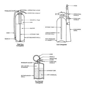
Examples of Water type, CO2 and Dry Chemical extinguishers
