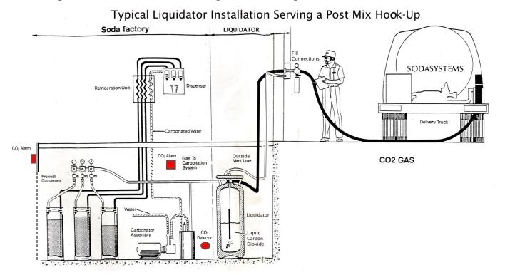
A post-mix fountain beverage dispensing system is defined by delivering a heavy concentrated beverage base and a diluent for the concentrated syrup to a dispense nozzle, adding one or more of colors, flavors and any additives to the beverage base and diluent to provide a completed carbonated beverage, and delivering this drink
