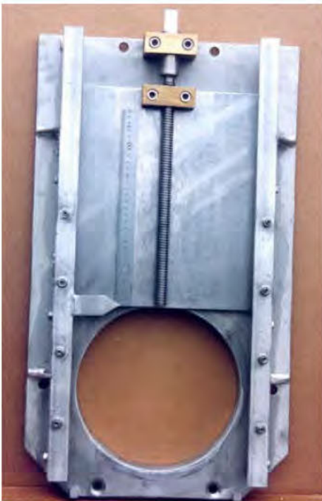
Example of an Orifice Gate
