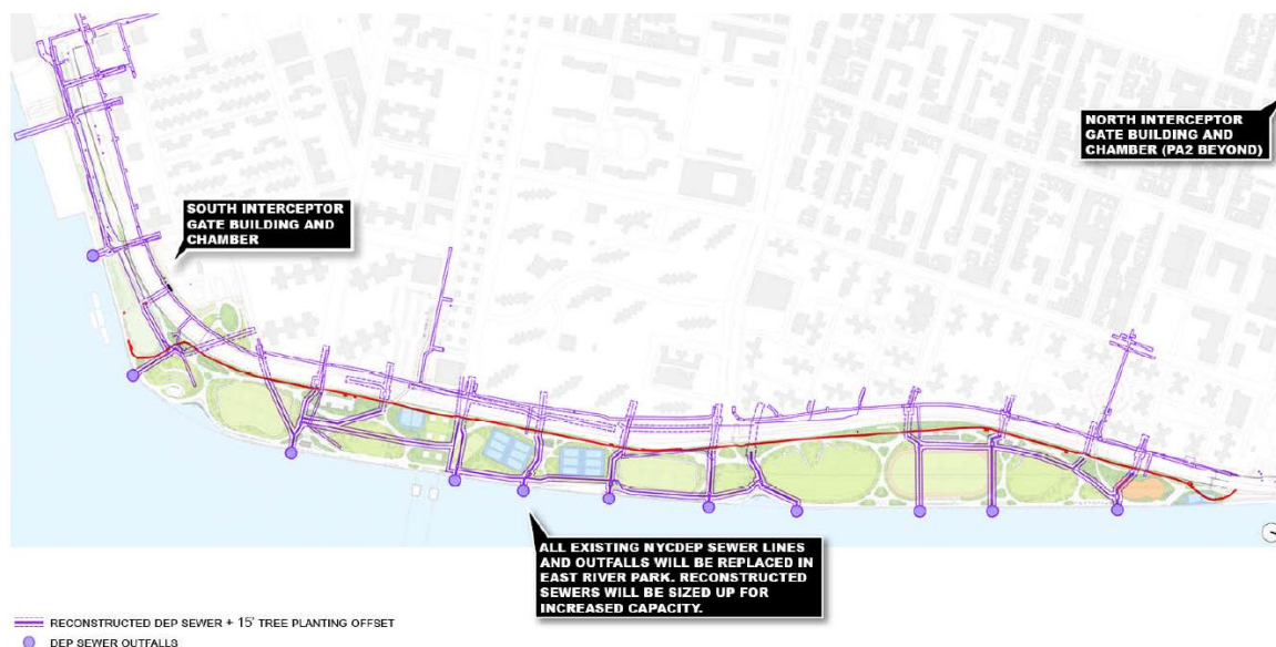
Figure 7: Sewer reconstruction works to improve drainage in East River Park. Source: East Side Coastal Resiliency Project Briefing with City Agencies, MBPO and Deltares. Manhattan Borough President’s Office, Sep 13, 2019.
