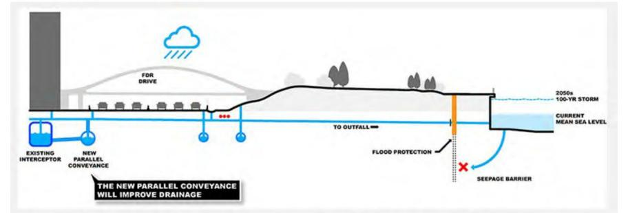
Upgrades to the combined sewer system are referred to here as Parallel Conveyance. These improvements will protect the inland neighborhoods on Manhattan's East Side from flooding due to rainfall.
