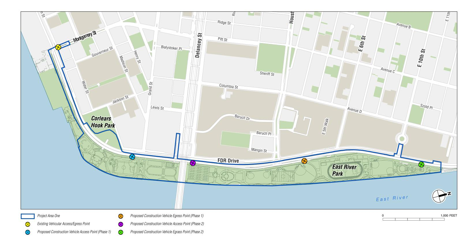
Existing and Proposed Construction Vehicle Access/Egress Points Figure 1 Attachment A FDR Drive Slip Ramp Traffic Study
