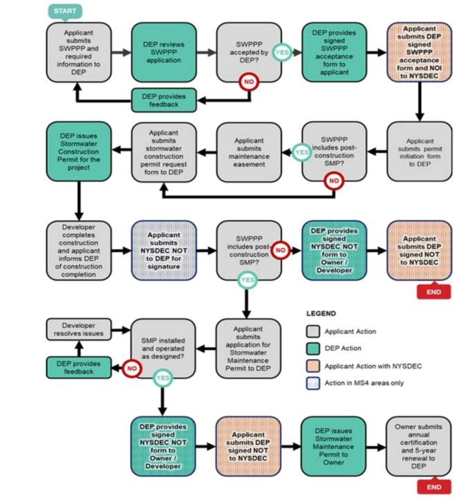
*Flow diagram #5:* detailed process for stormwater construction permits
