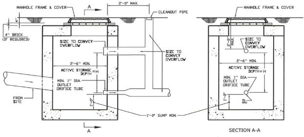
Figure F.5. Detention Tank with Re-Entrant Orifice
