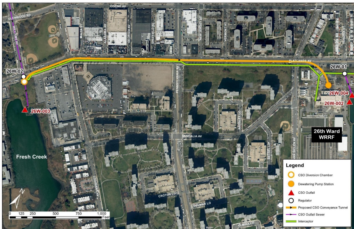
Figure 8-30. Layout of CSO Storage Tunnel and Dewatering Pumping Station at the 26 th Ward WRRF
