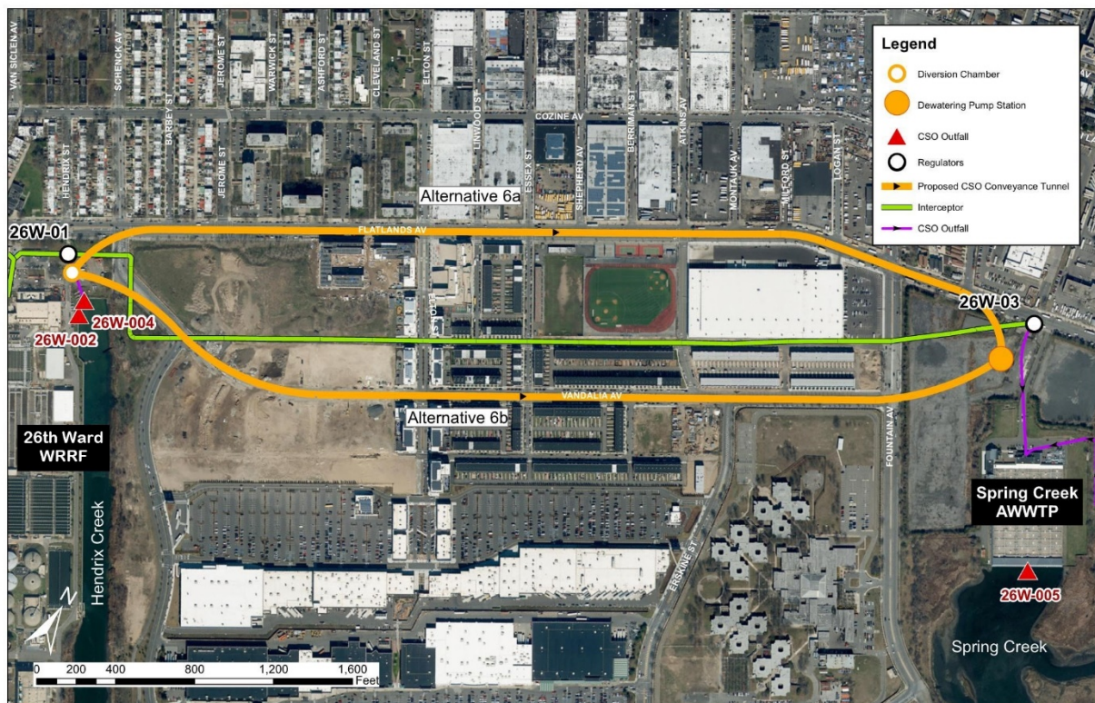
Figure 8-28. Layout of CSO Storage Tunnel and 50 MGD Dewatering Pumping Station at the Spring Creek AWWTP
