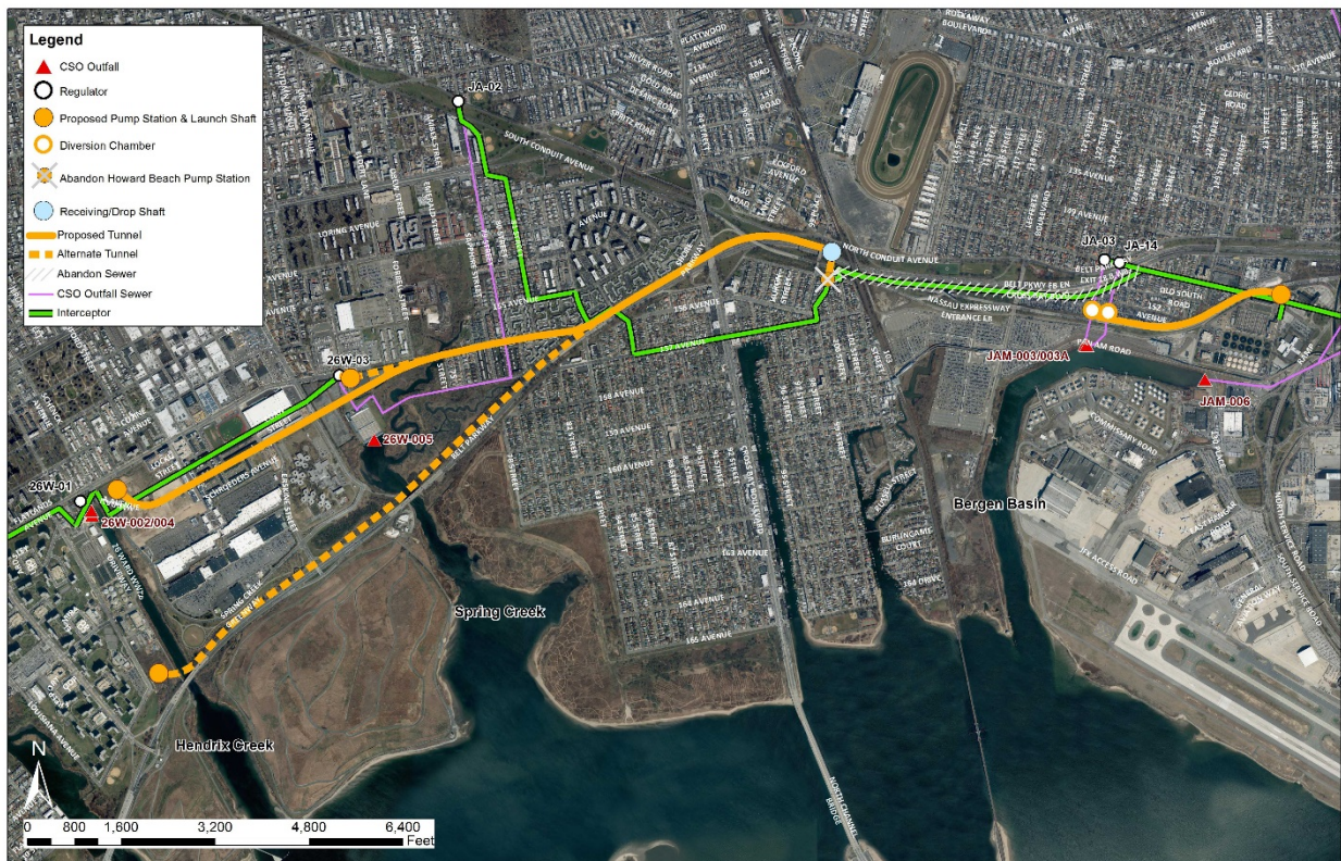
Figure 8-9. Layout for Proposed Parallel Interceptor to Jamaica WRRF and Gravity Sewer to 26 th Ward WRRF
