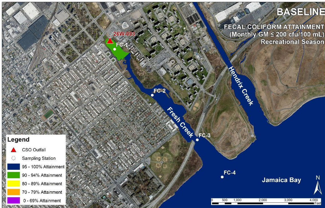
Model Predicted Fecal Coliform Recreational Season WQ Attainment for Fresh Creek Monitoring Station FC1
