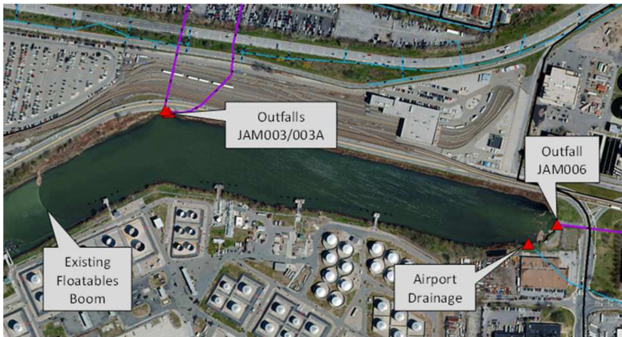
Figure 9. Location of Outfalls Relative to Existing Containment Boom in Bergen Basin
