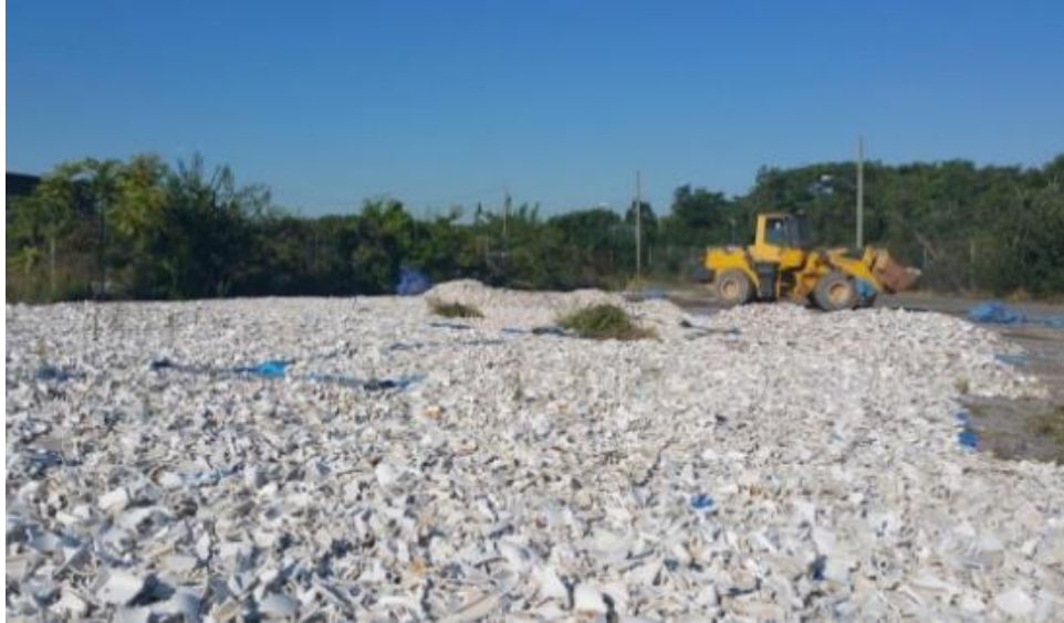
Figure 6-8: Crushed Porcelain used in Receiver Reefs
