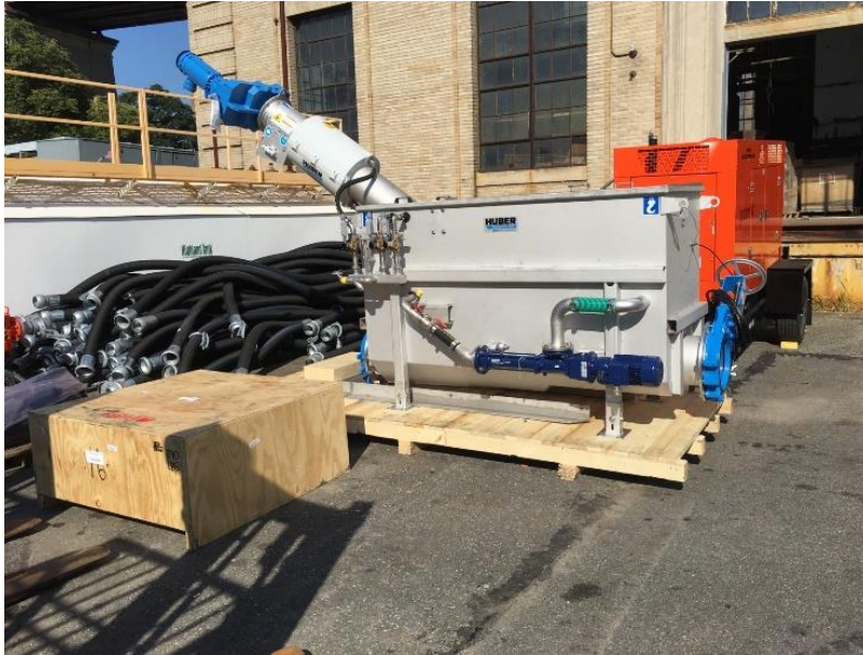
Figure 5-20: Huber ROTATMAT RPPS Pro- Rotary Drum Screen and Control Panel
