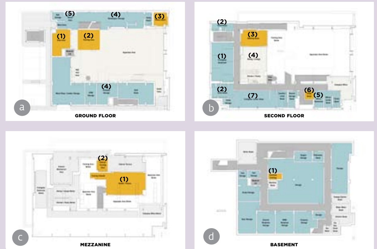
For Rescue Company 3, an array of program spaces were developed to meet the needs of the company. The ground floor (a), consists of a housewatch (a3), shop (a1), and training (a2) spaces. It also includes large spaces for storage (a4) and a deacon area (a5). The second floor is comprised of a firefighter bunkroom (b1), restrooms (b2), a meeting room (b3), a large dining and
