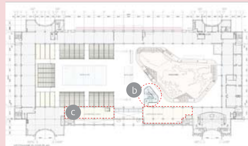
The ground level floor plan, above (top), focuses on the seven new galleries that ring the perimeter of the interior space. These galleries will provide space for many of the museum’s temporary exhibitions. The ceiling of each gallery is louvered, which allows
