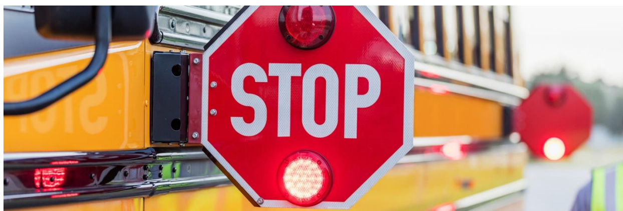
Figure 15. LED-Lighted Stop Arm (SeekingAlpha)
