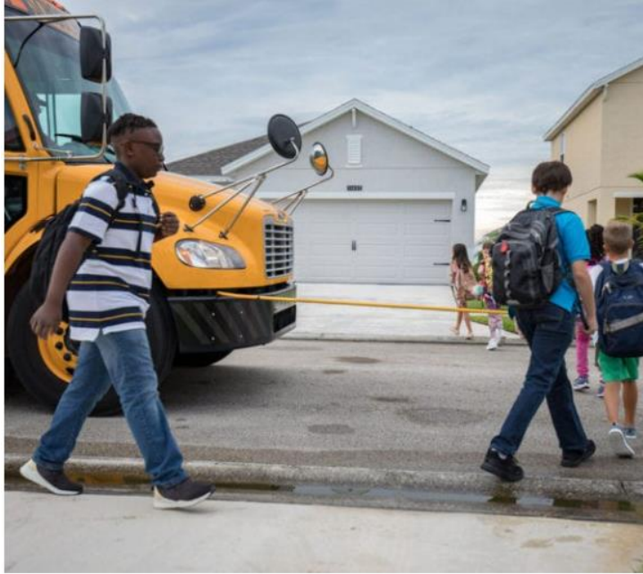
Figure 13. Crossing control arm (SafeFleet)
