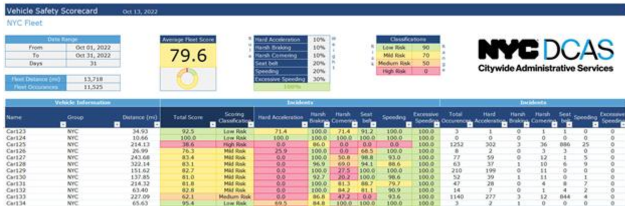
Figure 32. Example driver safety scorecard based on telematics reporting on NYC municipal fleet (NYC DCAS)
