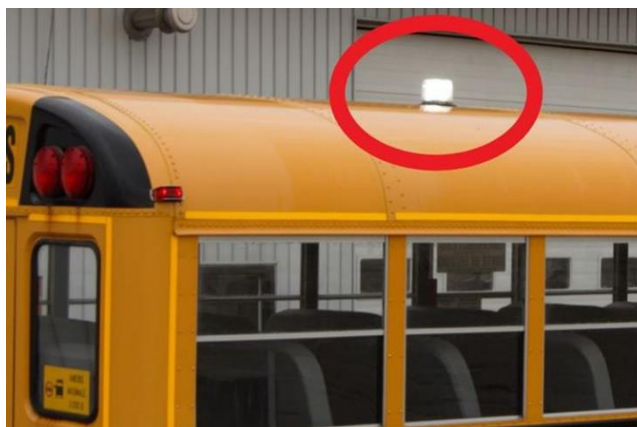
Figure 16. Roof-Mounted Strobe Light (Durham Radio News)
