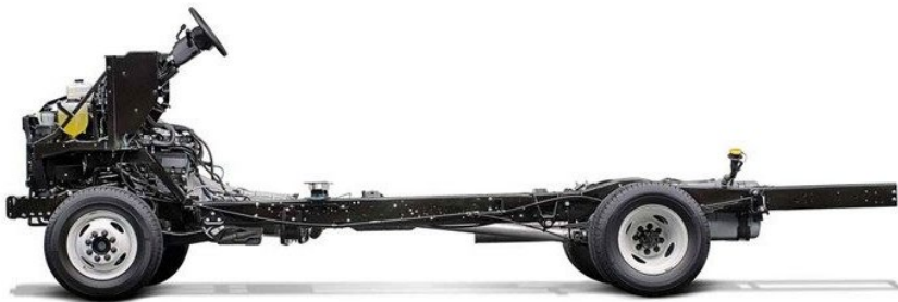
Figure 5: Ford E350 Stripped Chassis (Source: alpackerford.net)
