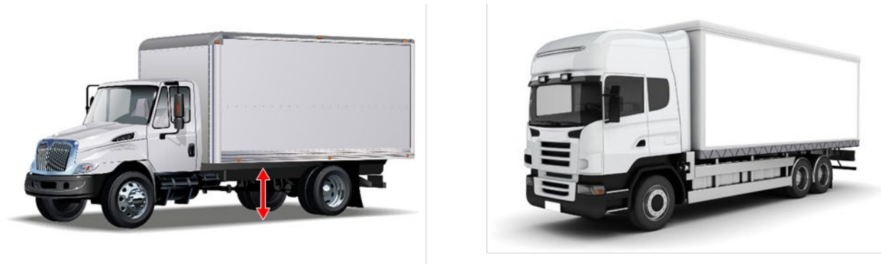
Figure 1. Picture. Side-by-side comparison of trucks with and without LPDs, with the unshielded gap between axles marked by a red arrow.
