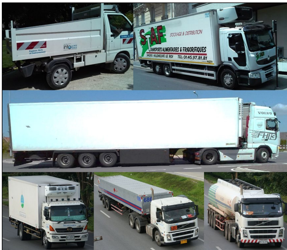
Figure 2. Photographs. Images of UN Regulation 73 LPDs in France (top), the Netherlands (middle), and Thailand (bottom).
