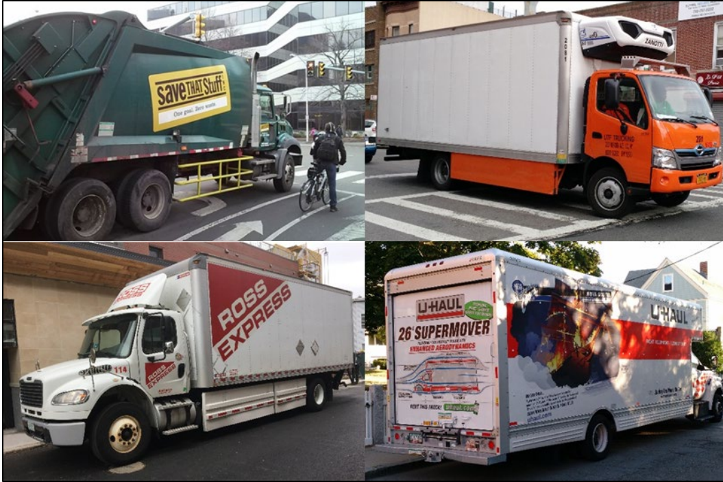
Figure 16. Photographs. Private sector rail and panel style LPDs in the Boston and New York City metro areas.
