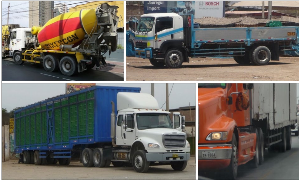
Figure 9. Photographs. Single-unit and combination tractor trailers equipped with LPDs in Peru Source: Volpe.
