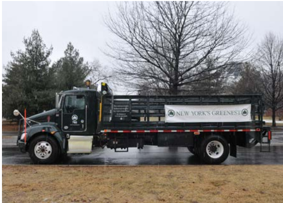
This Parks and Recreation Department hybrid diesel electric rack truck operates on B20. – Photo courtesv of New York Citv
