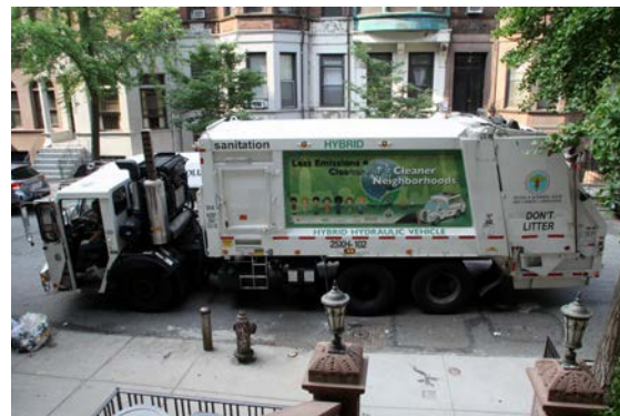
A Sanitation Department hybrid hydraulic garbage truck also operates on B20. – Photo courtesy of New York City
