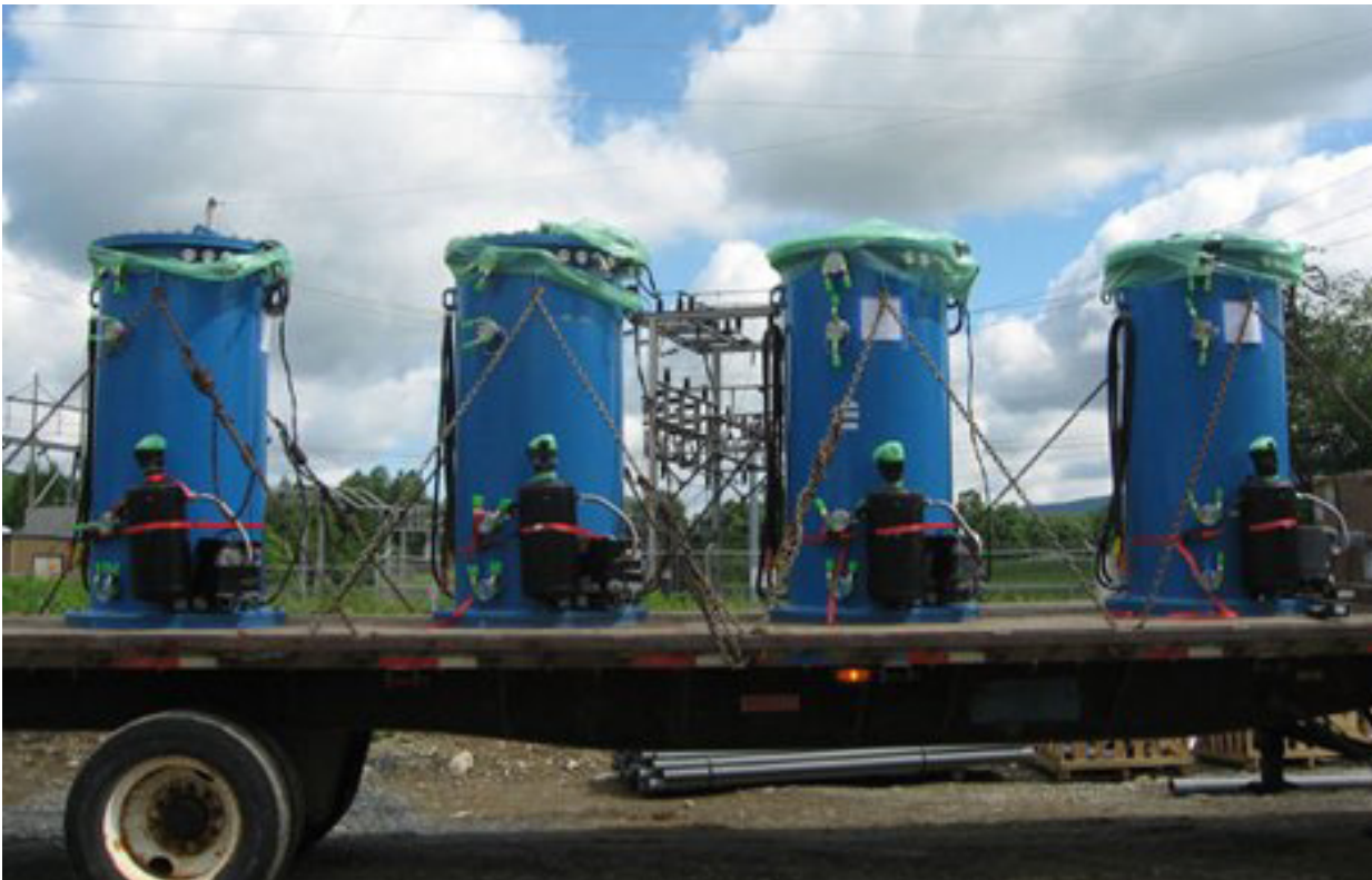
Figure 5: Flywheel Energy Storage Technology 11
