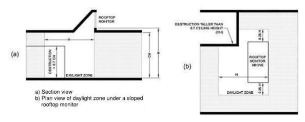
FIGURE C405.2.3.2(3) DAYLIGHT ZONE UNDER A SLOPED ROOFTOP MONITOR
