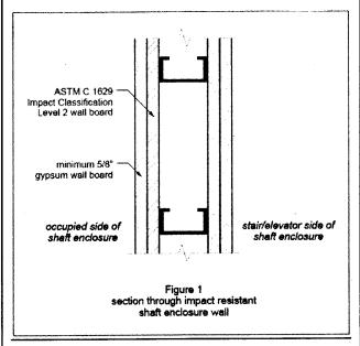
Assembly. The wall assembly shall be at least two-hour fire resistance rated.
