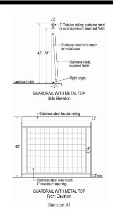
All guardrail components and hardware shall be in No. 316 Stainless Steel, passivated and bead blasted.
