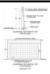
All guardrail components and hardware shall be in No. 316 Stainless Steel, passivated and bead blasted.
