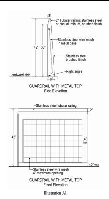
All guardrail components and hardware shall be in No. 316 Stainless Steel, passivated and bead blasted.
