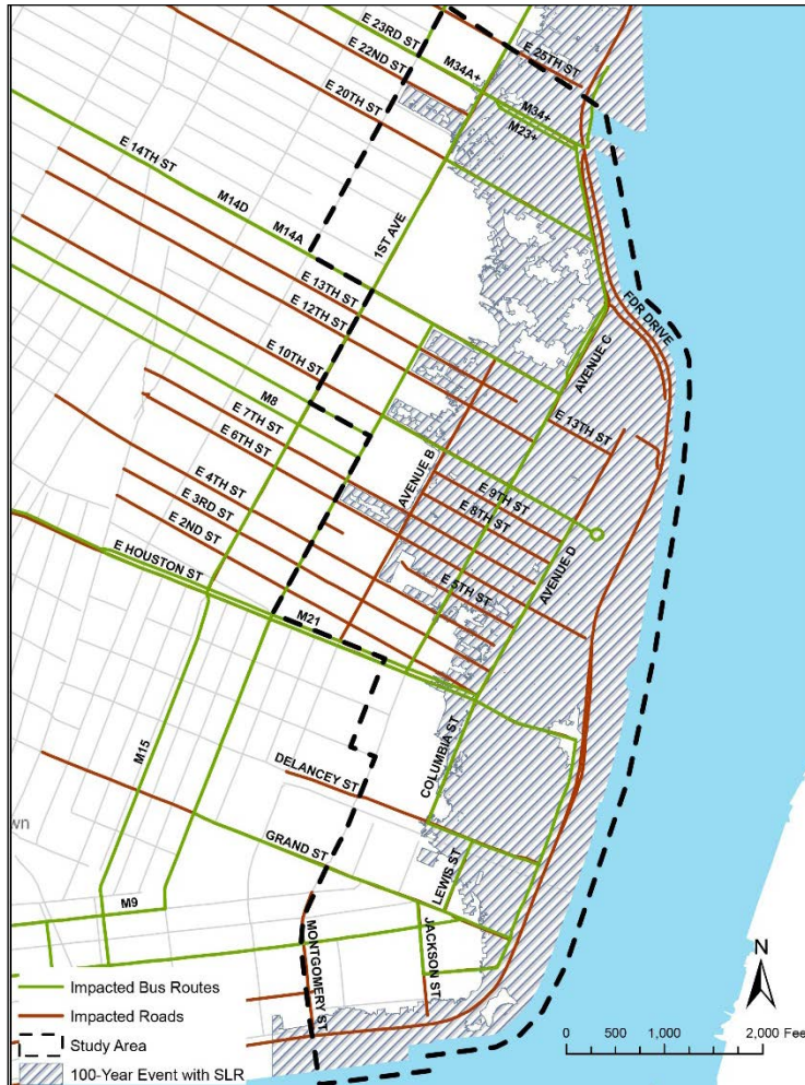
Figure 12. Impacted Streets During the 1 Percent Annual Chance Coastal Surge Event, Plus SLR in the 2050s
