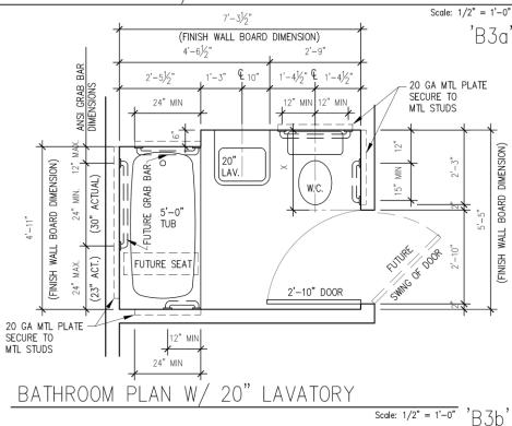
X = THE OUTER EDGE OF THE WATER CLOSET WILL NOT EXTEND INTO THE CLEAR SPACE REQUIRED FROM THE DOOR OPENING.
