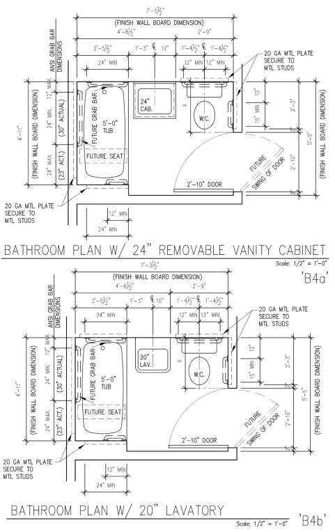
X = THE OUTER EDGE OF THE WATER CLOSET WILL NOT EXTEND INTO THE CLEAR SPACE REQUIRED FROM THE DOOR OPENING.
