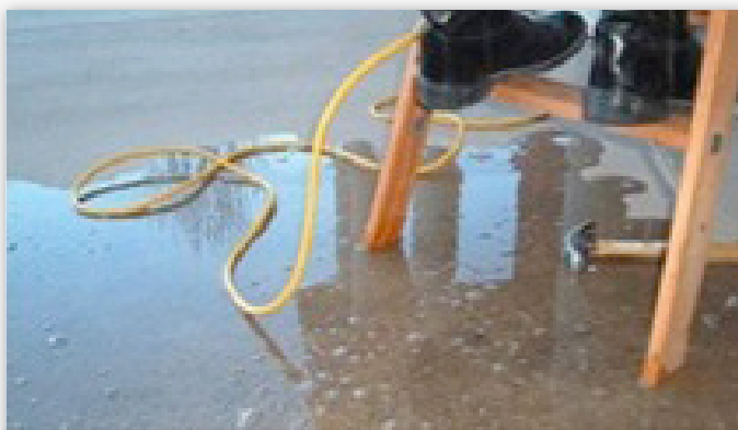
Don't allow extension cords to lay in water or solvents
