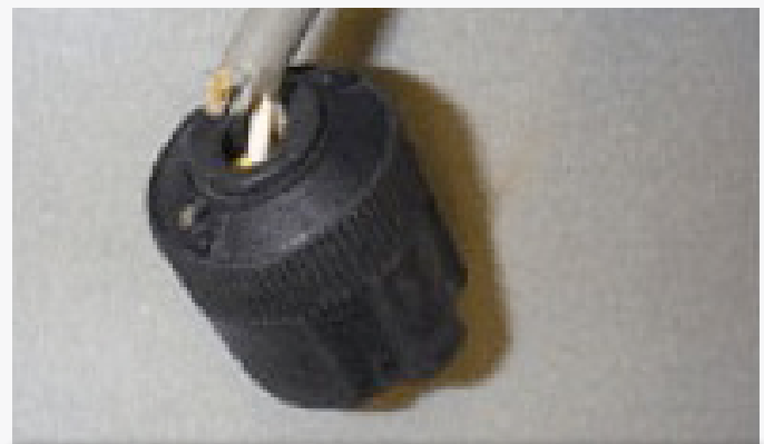
Defective cords with cuts through the insulation or with damaged ground prongs can cause shocks
