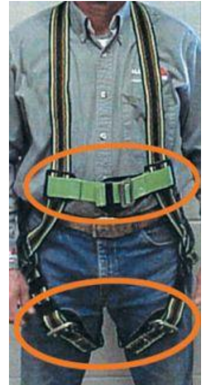
Chest strap positioned incorrectly. Should be located at mid-chest to keep shoulder straps snug. Leg straps are too loose.
