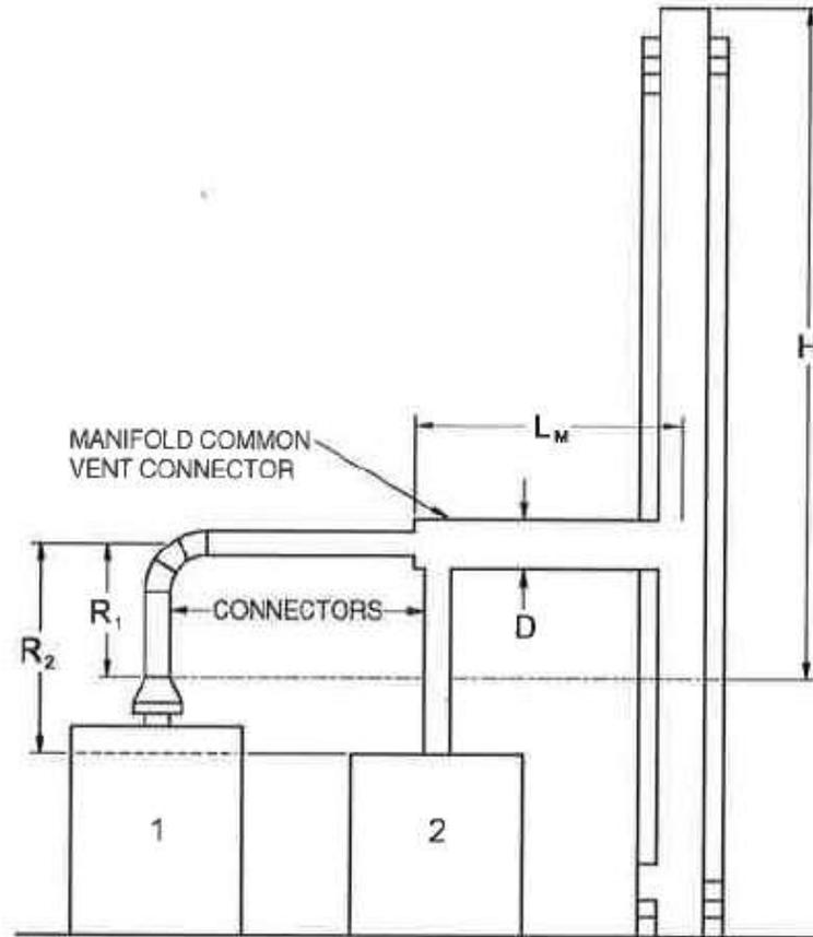
Example: Manifolded Common Vent Connector  $L_M$  shall be no greater than 18 times the common vent connector manifold inside diameter; i.e., a 4-inch (102 mm) inside diameter common vent connector manifold shall not exceed 72 inches (1829 mm) in length (see Section 504.3.4).
