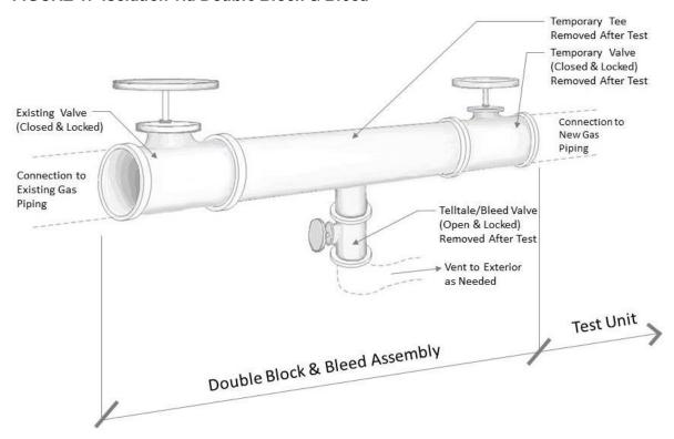
NOTE: In addition to the fabricated assembly shown in FIGURE 1, a single unit manufactured as a double block and bleed may be used for testing. Such unit shall be used in accordance with the manufacturer's specifications and rating.
