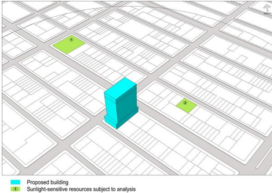
FIGURE 8-7 - THREE-DIMENSIONAL COMPUTER MODEL SET UP FOR TIER 3 SCREENING ASSESSMENT
